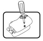
5. Replace the battery cover and tighten the screw to secure.
